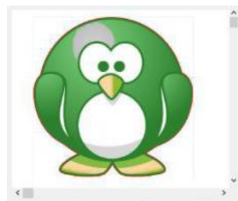
Preview of trace after Blackout is checked. The internal red cut lines are removed.
