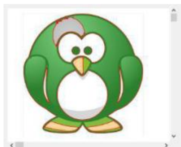
Preview of trace with Blackout not checked. Note the internal red lines that would be cut.
